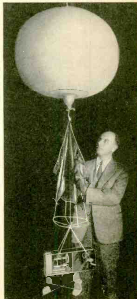
We recently described a European S-W transmitter sent up, attached to a balloon, for signaling the upper air conditions to weather observers. This photo shows similar apparatus used by the U. S. Weather Bureau.
